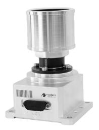
The Auriga™ star tracker, with its standardized components, is specifically designed to meet cost reduction objectives while offering excellent technical performance and reliability. Auriga™ is the legacy of 50 years of Sodern experience in space equipment development and the Hydra high-performance star trackers. Auriga™ offers fast acquisition of about 3 seconds for an accuracy of 5 arc seconds.
